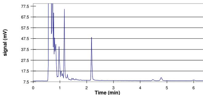
To the left is a chromatogram of a sample collected in an evacuated cannister at waist level while fueling a vehicle. The cannister was subsequently filled to 42 pounds with dry lab nitrogen which translates to approximately a 3X dilution of the sample. This sample was also analyzed using the 30 microliter loop injection.
